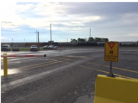
*barricades can protect stationary employees as well as guide them to a desired route, signage warns of exits leading into traffic areas.
